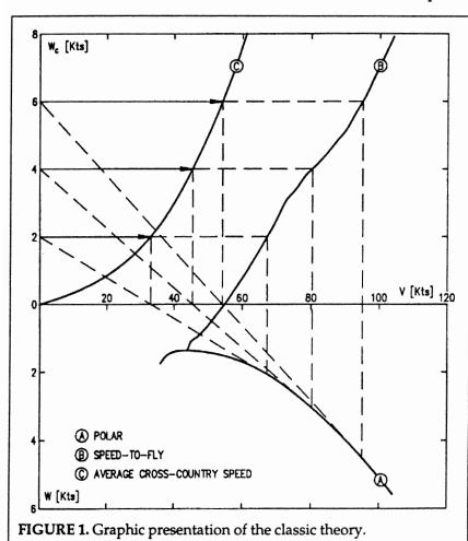
If the air between the updrafts moves vertically, the polar curve will be shifted up or down, and the shift will be equal to the vertical speed of the air mass  $W_{\rm w}$ . ( $W_{\rm w}$  is assumed positive when the air moves upward.) In this case, equation (1) should be adjusted by substituting  $W_{\rm g}$  with  $W_{\rm g}$ -  $W_{\rm w}$ . The optimum cruising speed can be obtained from the still air speed-to-fly curve, by subtracting  $W_{\rm w}$  from the rate of climb  $W_{\rm c}$ .
