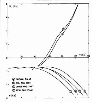
**FIGURE 6.** Polar shift in a 40 kt wind ( $\beta = 110^{\circ}$ ;  $C_{ud} = 0$ ).
