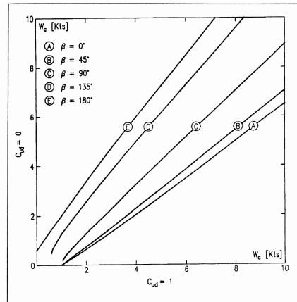
**FIGURE 9.** Break-even curves for 25 knot wind, Discus, W/S = 7.63 lb/ft, h = 3000 ft.
