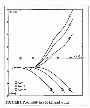
In a more general case, the updraft horizontal movement can be anywhere between zero and the full wind speed ( $0 \le C_{ud} \le 1$ ). To obtain the optimum speed-to-fly, we will again measure the glider horizontal speed in the
