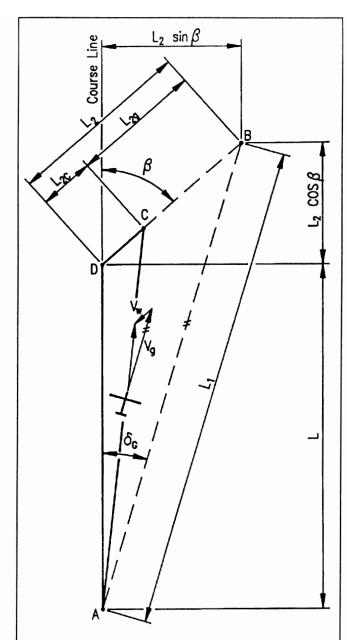
FIGURE 7. Cruise-climb cycle in ground reference system.
