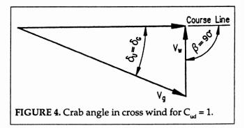
Viewed from the updraft reference system, the polar shift now depends not only on the wind speed, but also on the cruising speed of a glider:
